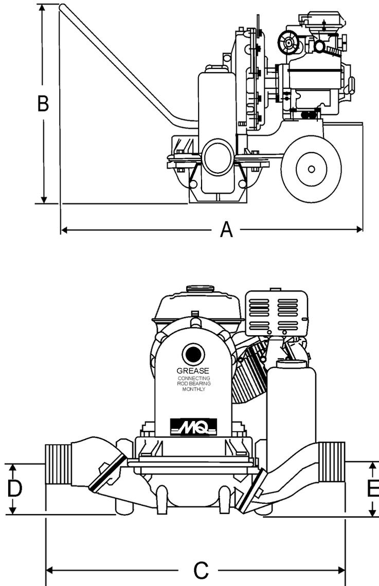
Figure 1. MQ-D206HPump Dimensions
