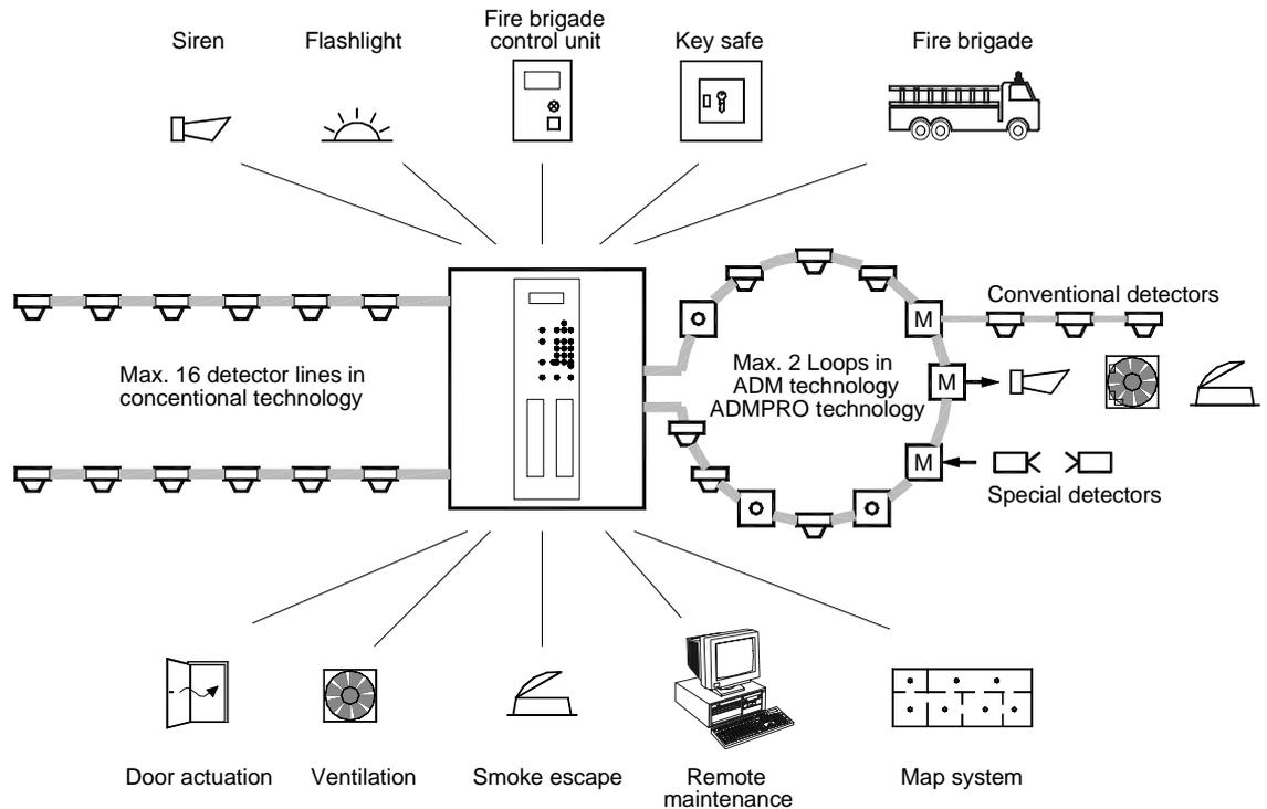
Figure 2: View of a typical fire detection system constructed with the fire detection control panel BC216-1
