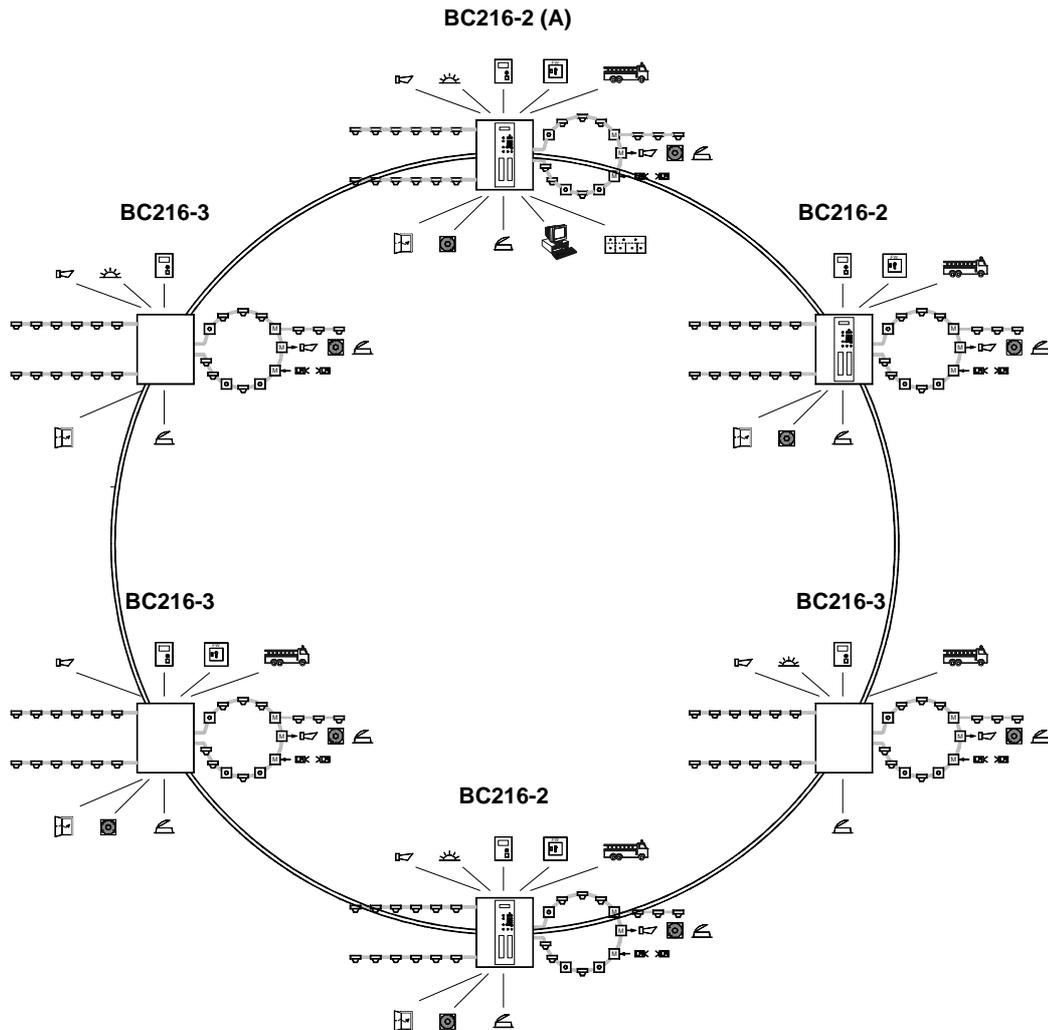
Figure 3: View of a typical fire detection system constructed with the fire detection control panel BCnet216
