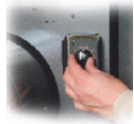
Use the High Idle (OCV) engine speed adjustment dial to change the heat input to the arc:
