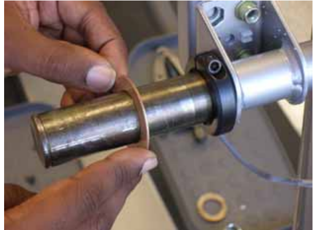
Fig 6: Installing the Oilite washer
