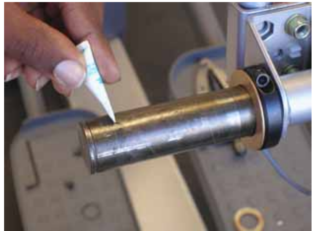
Fig 7: applying Loctite to the deadshaft
