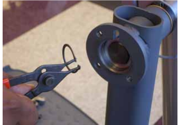
Fig 12: installing the snap ring
