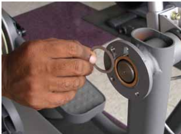
Fig 11: installing the thrust washer
