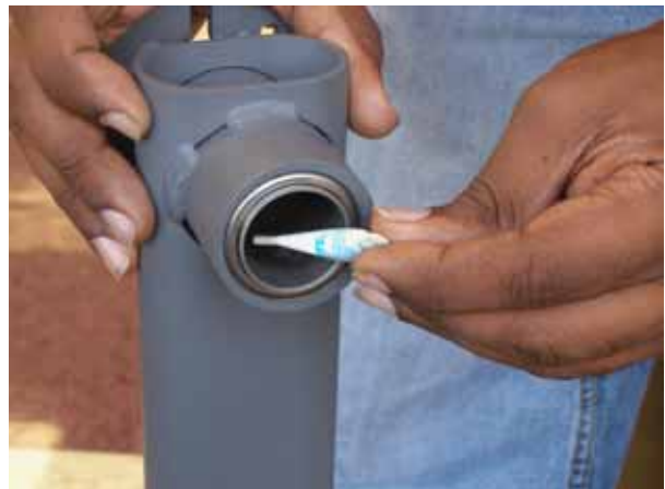
Fig 8: applying Loctite to the rocker arm
