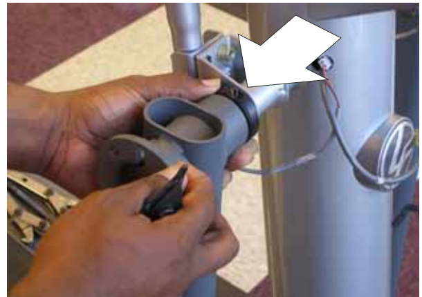
Fig 13: pull the shaft collar in the direction of the arrow
