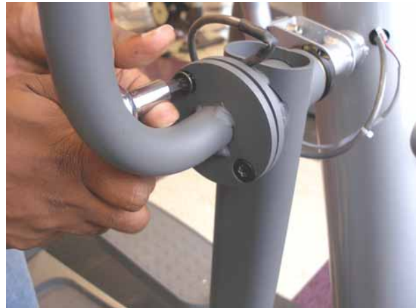
Fig 1: removing the user arm
