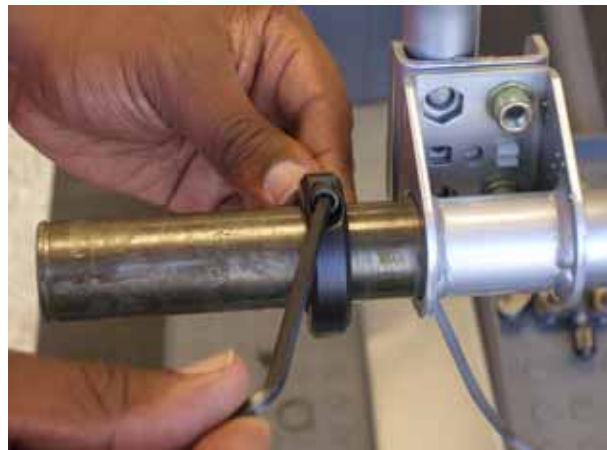
Fig 4: loosening the shaft collar
