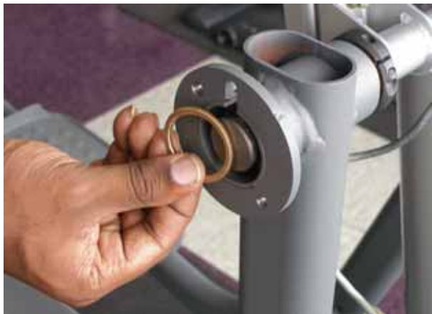
Fig 10: installing the Oilite washer
