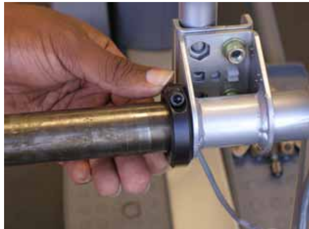
Fig 5: slide the collar against the bullhorn bracket
