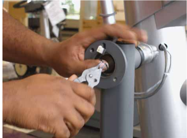
Fig 3: removing the snap ring from the deadshaft
