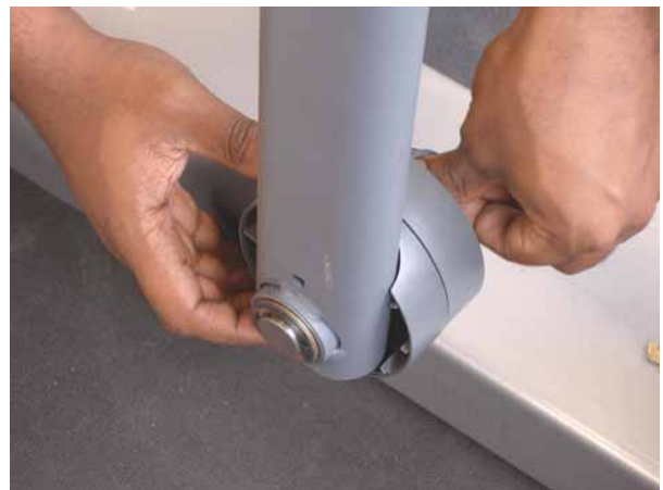
Fig 2: separating the pedal from the rocker arm
