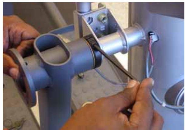
Fig 14: tightening the shaft collar
