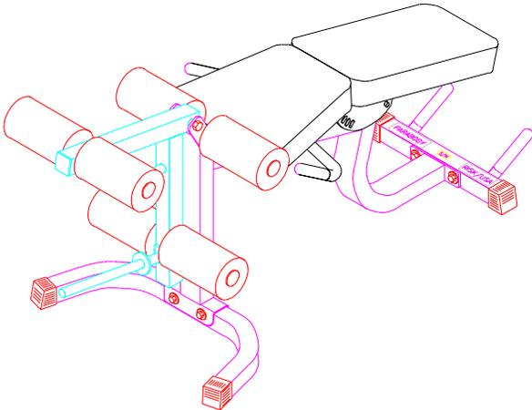
**STEP 1:** Insert four PARABODY LOGO END CAPS (37) into the ends of REAR BASE LEG (12) and FRONT BASE SUPPORT (1). See FIGURE 1.
