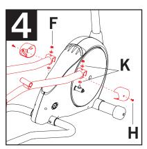
STEP 4: ATTACH LEFT & RIGHT PEDAL ARMS AND PEDAL ARM SLEEVES.
