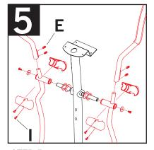
STEP 5: ATTACH LEFT & RIGHT LOWER HANDLE BARS TO CONSOLE MAST. ATTACH LEFT & RIGHT UPPER HANDLE BARS. ATTACH H-BAR COVERS. Note: Bolts and washers are pre-assembled.
