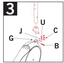
STEP 3: ATTACH CONSOLE MAST AND CONSOLE MAST BOOT.
