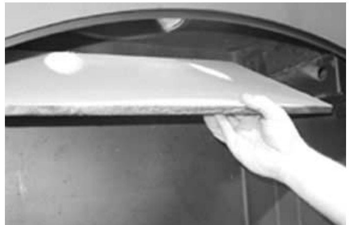
Figure 31B-Removing Baffle shown without ceramic blanket
