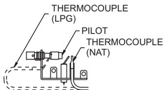
for about one (1) minute after the pilot is lit. Release knob and it will pop back up. Pilot should remain lit. If it goes out, repeat steps 2 through 6.
