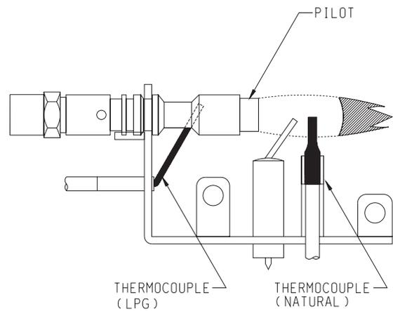
**Incorrect Flame Pattern for VFDT & VFDM**
