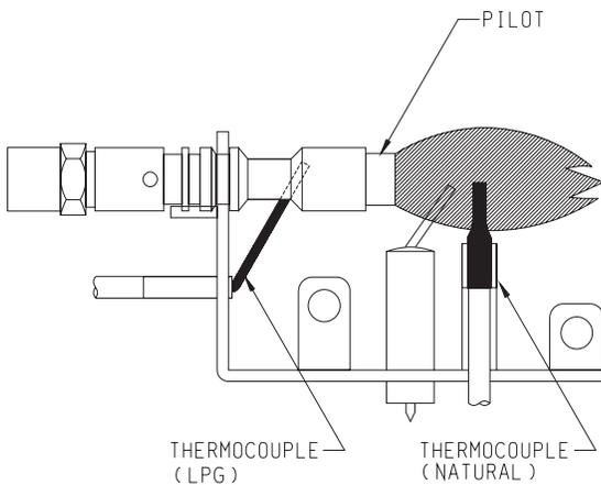
**Correct Pilot Flame Pattern for VFDT & VFDM**
