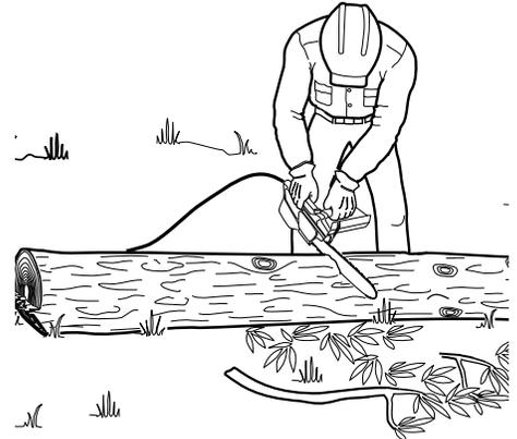
Figure 13 - Bucking Log With Entire Length On Ground
