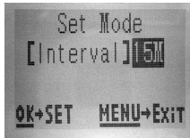
(Schritt 7)- Field Scan-Intervall festlegen
