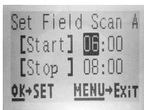
[Step 3]-set Field Scan “A” Stop & Start
