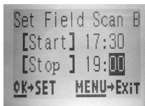
[Step 5] (opt)-set Field Scan “B” Stop & Start
