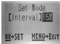
[Step 7]-set Field Scan Interval
