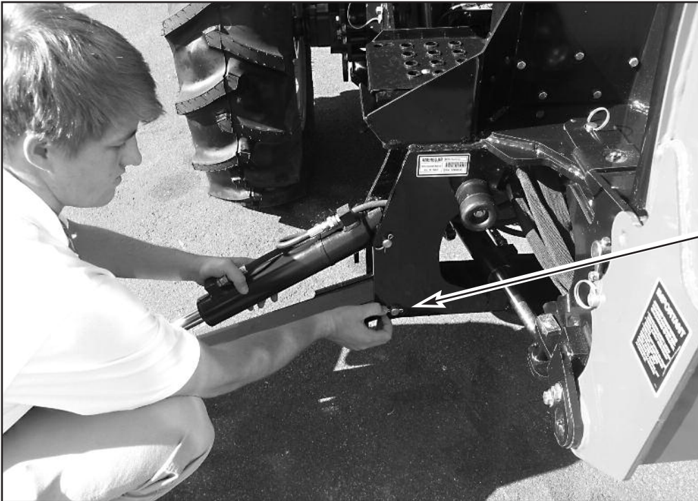
Pinning Stabilizer Into Place
