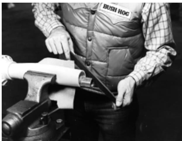
M. Apply multi-purpose grease to inside of outer (female) driveline section. Assemble driveline and install on tractor and cutter. Pull on each driveline section to be sure yokes lock into place. Make certain driveline shielding is in place and in good condition.
