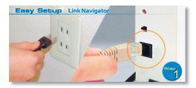
Connect the other end of the Ethernet Cable into a hub, switch, or router on the network, or connect it directly to a PC. Connecting directly to a PC is not recommended. Many features, including DHCP, will not work when LinkStation is connected directly to a PC.
