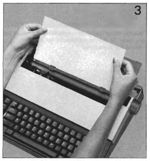
When the paper comes between the platen and the paper bail scale, return the paper bail scale to its original position. In order to adjust the paper, push the paper release lever (which loosens the paper) and make necessary adjustments.
