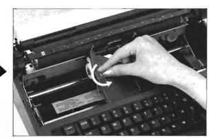
Turn the ribbon feed knob counterclockwise to take up any slack. (To remove the cassette ribbon, simply reverse this procedure.)
