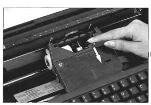
Pull the green motor lock lever on the carrier toward you.
