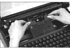
To insert a cassette ribbon, turn the ribbon feed knob on the cassette counterclockwise to tighten the ribbon. Then use both hands to slip the back edge of the cassette onto the carrier.
