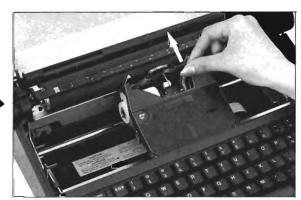
Press the motor lock lever toward the platen until it clicks into place. Do not force the lever. If you have difficulty, check again to see that the daisy wheel is set properly.
