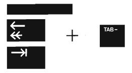
Use the space bar and backspace key, or the TAB key as required to bring the carrier to the position at which you desire to clear a tab. Then press the TAB — key to clear the tab.
