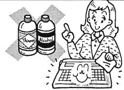
Never use volatile liquids such as thinner or benzine to clean the exterior surface of the typewriter. Use only a soft cloth dampened with a mild detergent solution.
