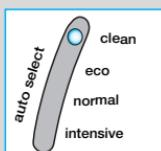
When the program is finished, the blue «clean» light will shine. You can release the shaver by pushing the «start cleaning» button.
