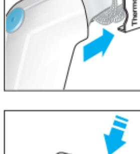
1. To achieve accurate measurements, make sure a new, clean lens filter (2) is in place before each measurement.
