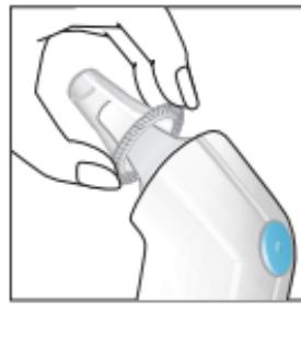
5. For the next measurement, remove the used lens filter and put on a new, clean lens filter. Clear the display by pushing the «start» button once. Fit the probe snugly into the ear canal, then push the «start» button.
