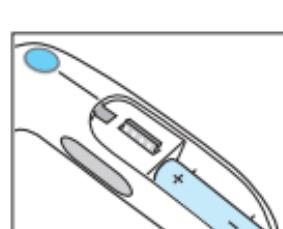
The thermometer is supplied with one 1.5 V type AAA (LR 03). For best performance, we recommend Duracell® alkaline batteries. Insert new battery when the battery symbol appears on the display.
