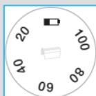
The shaver display (16) shows the charge status of the battery. During charging or when using the shaver, the respective green charge status will blink. When the battery is fully charged the green charge status will light up continuously, provided the shaver is switched on or connected to an electrical outlet.
