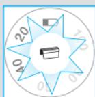
The replacement symbol will remind you during the next 7 shaves to replace the Foil & Cutter cassette. Then the shaver will automatically reset the display.
