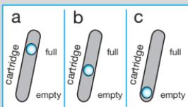
The display for cleaning fluid (6) will show how much cleaning fluid is in the cartridge:
