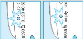
Model 8590: When the shaver is fully charged, all five green charging lights (16) will light up (20% per light), provided the shaver is connected to an electrical outlet or switched on.
