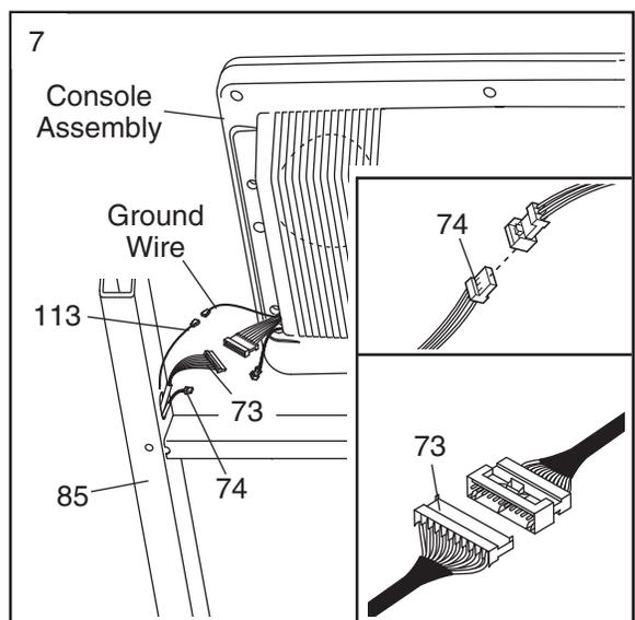
8. Set the console assembly on the Uprights (85). **Make sure that no wires are pinched.** Finger tighten a Console Bolt (72) with a Star Washer (67) into the lower hole in each Upright (only one side is shown).
