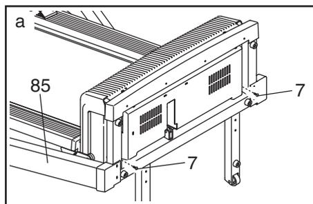
b. Raise the Uprights (85) to the vertical position. Remove the three Screws (7) from the Hood (33), and carefully pivot the Hood off.
