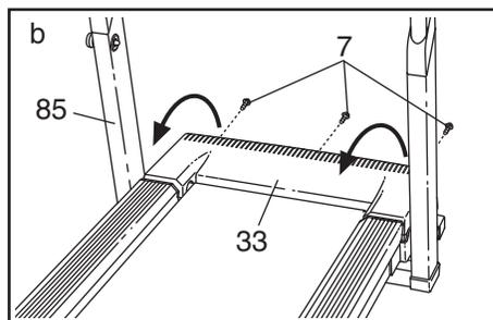
Locate the Reed Switch (22) and the Magnet (18) on the left side of the Pulley (17). Turn the Pulley until the Magnet is aligned with the Reed Switch. **Make sure that the gap between the Magnet and the Reed Switch is about 1/8".** If necessary, use a slotted screwdriver to move the Reed Switch slightly. Reattach the Hood (33), making sure that the Screws (7) are inserted into the same holes from which they were removed. Run the treadmill for a few minutes to check for a correct speed reading.
