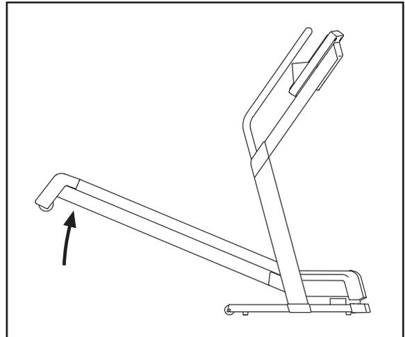
2. Move your right hand to the position shown and hold the treadmill firmly. Using your left hand, pull the latch knob to the left and hold it. Raise the treadmill until the latch pin is aligned with the indicated hole in the frame. Insert the latch pin into the hole. **Make sure that the latch pin is fully inserted into the hole.**
