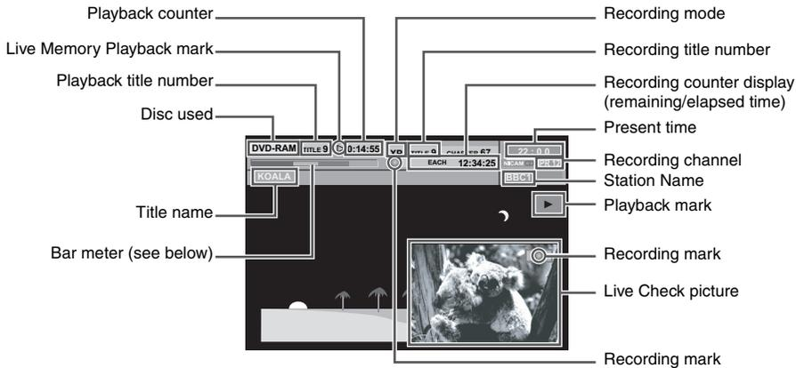
This unit displays the current recording/playback status by the bar meter.
