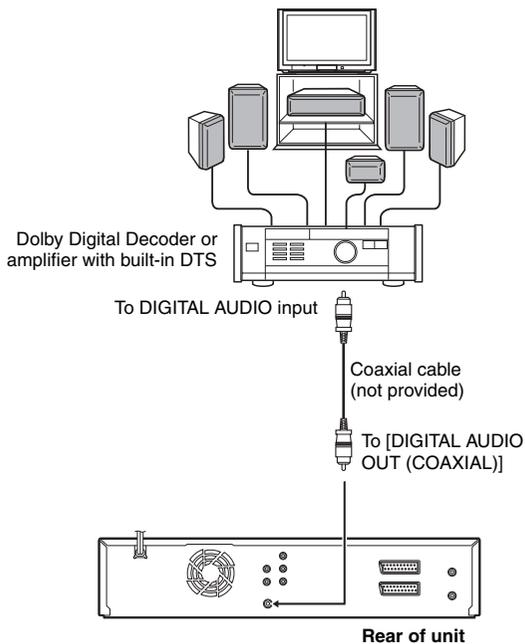
**1** Connect the unit and a Dolby Digital Decoder or an amplifier with built-in DTS using an optional coaxial cable.
