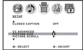
**2** Press ◀ or ▶. The PICTURE SIZE menu will appear. Press ▲ / ▼ or a **Number button (0-4)** to select the desired picture size, as described below and on the next page, then press **ENTER**.
