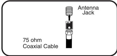
For basic Cable TV service not requiring a Converter/Descrambler box, connect the 75 ohm Coaxial Cable directly to the Antenna Jack on the back of the TV/DVD.
