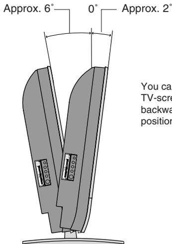
You can adjust the angle of the TV-screen up to 2° forward or 6° backwards from the vertical position.
