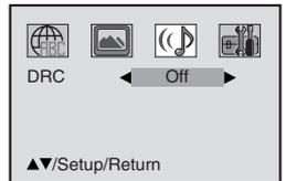
**On** : Loud sound such as explosion or similar is toned down slightly when play back. This makes it suitable for when it is connected to a stereo.
