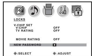
**5** Enter a new password using **Number buttons (0-9)**, then press **ENTER**.
