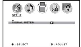
3 Press ◀ or ▶ to check the Digital-signal strength.
