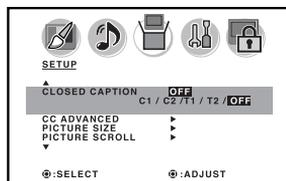
When a Digital signal is received, you can choose from CS1, CS2, CS3, CS4, CS5, CS6, C1, C2, C3, C4, T1, T2, T3, T4 and OFF.
