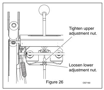
If chute does not rotate freely:
