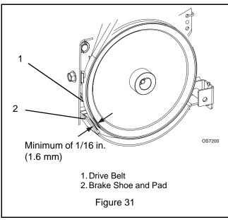
4. Repeat steps 1 − 3 until spring extension and brake clearance are within specified range.
