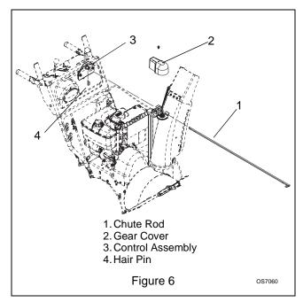
Use the handlebar hardware locations on the side of the unit frame to determine which hole gets used to secure the chute rod to the control assembly.
