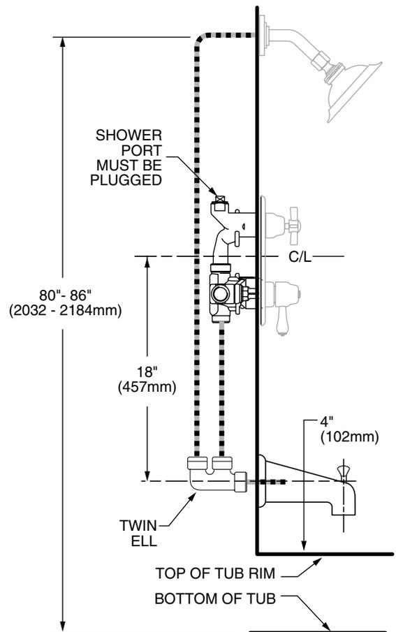
**IMPORTANT: WHEN NOT USING A DIVERTER SPOUT A SEPARATE DIVERTER VALVE MUST BE USED.**
