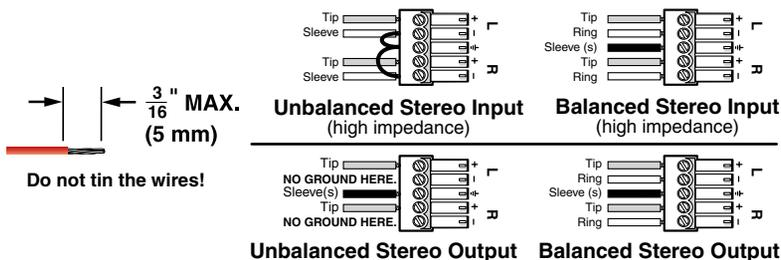
**CAUTION** For unbalanced audio output, connect the sleeve(s) to the ground contact. **DO NOT** connect the sleeve(s) to the negative (-) contacts.
