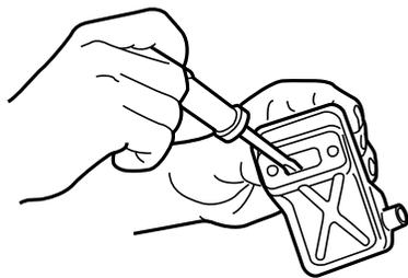
1. Remove the muffler, insert a screwdriver into the vent, and wipe away any carbon buildup. Wipe away any carbon buildup on the muffler exhaust vent and cylinder exhaust port at the same time.
