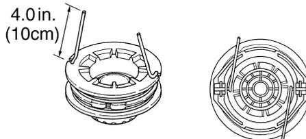
6. While holding the spool against the housing, pull the line ends to release them from the slot.
