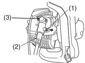
2. Pull out the inner shaft from the clutch housing side hole, apply Zenoah Guine Power Grease (Z3180-91250) or lithium-based heat-resistant grease (#2) to the shaft, and insert the shaft back into the liner.
