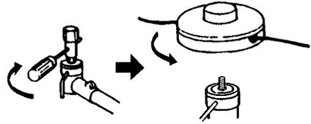
1. While locking the gear shaft, by inserting the supplied tool into the upper holder on the gearbox, loosen and remove the hexagon nut (left-handed).
