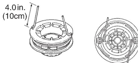
6. While holding the spool against the housing, pull the line ends to release them from the slot.
