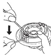
7. Line up the slot on the bottom cap with the hook on the housing, press the cap against the housing until it clicks.
