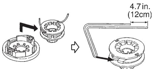
4. Wind up the line in the correct direction as indicated on the spool.
