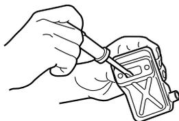
1. Remove the muffer, insert a screwdriver into the vent, and wipe away any carbon buildup. Wipe away any carbon buildup on the muffer exhaust vent and cylinder exhaust port at the same time.
