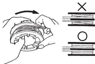
5. Hook each end of the line in the slot on the edge of the spool, and then put the ends through the eyelets on the housing. Make sure that the spring and the washers are in place.
