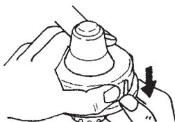
3. Take out the spool and pull off the old line. Put one end of new line through the spool holes and pull it until the length is equal between each part of the line.
