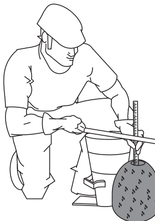
Figure 41-F. Slump Test (Measurement)
