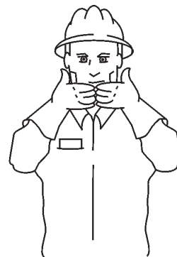
ALL DONE CLEAN-UP
