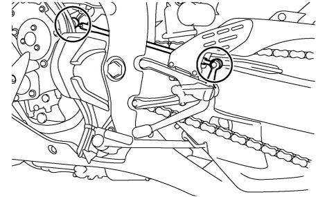
The operation of the shift pedal should be checked before each ride, and the shift pedal rod pivots should be lubricated if necessary.
