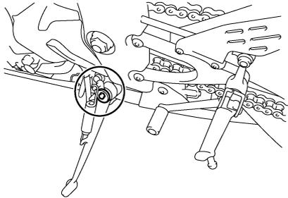
The operation of the sidestand should be checked before each ride, and the sidestand pivot and metal-to-metal contact surfaces should be lubricated if necessary.
