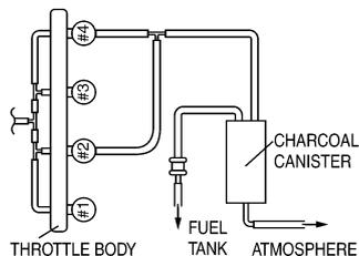
This model is equipped with a canister to prevent the discharging of fuel vapor into the atmosphere. Before operating this vehicle, make sure to check the following:
