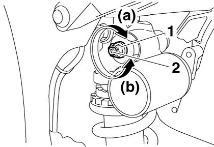
1. Compression damping force adjusting bolt (for fast compression damping)
