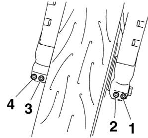
1. Front wheel axle pinch bolt A
