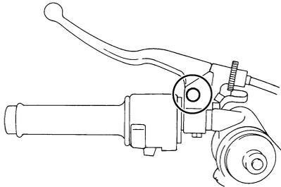
The operation of the brake and clutch levers should be checked before each ride, and the lever pivots should be lubricated if necessary.
