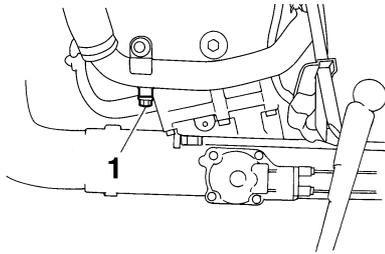
1. Coolant drain bolt
