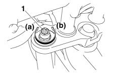
1. Spring preload adjusting bolt
