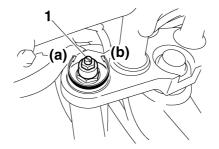
1. Compression damping force adjusting screw
