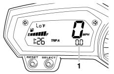
1. Odometer/tripmeter/fuel reserve tripmeter
