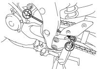
The operation of the brake and shift pedals should be checked before each ride, and the pedal pivots should be lubricated if necessary.
