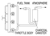
This model is equipped with a canister to prevent the discharging of fuel vapor into the atmosphere. Before operating this vehicle, make sure to check the following:
