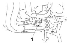
1. Engine oil drain bolt
