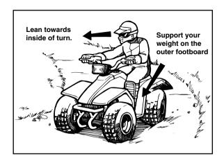
This procedure should be practiced at slow speed many times in a large off-road area with no obstacles. If an incorrect technique is used, your ATV may continue to go straight. If the ATV doesn't turn, come to a stop and then practice the procedure again. If the riding surface is slippery or loose, it may help to position more of your weight over the front wheels by moving forward on the seat.
