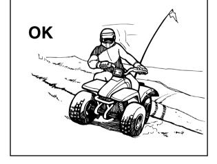
If your ATV has stalled or stopped and you believe you can continue up the hill, restart carefully to make sure you do not lift the front wheels which could cause you to lose control. If you are unable to continue up the hill, dismount the ATV on the uphill side. Physically turn the ATV around and then descend the hill.
