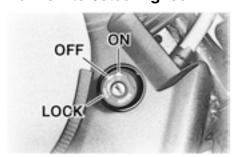
The main switch/steering lock controls the ignition and lighting systems, and is used to lock the steering. The various positions are described below.
