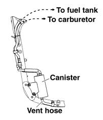
This model is equipped with a canister to prevent the discharging of fuel vapor into the atmosphere.
