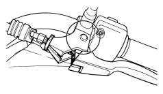
The operation of the brake and clutch levers should be checked before each ride, and the lever pivots should be lubricated if necessary.
