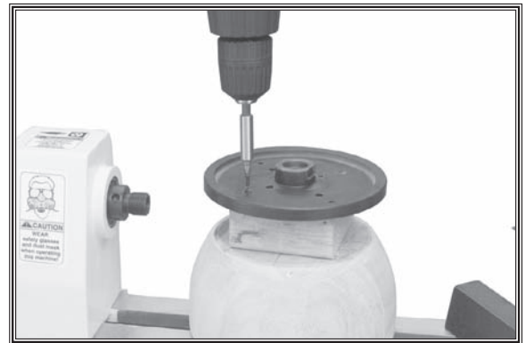
Figure 31. Typical attachment of faceplate to workpiece (shown with backing block).
