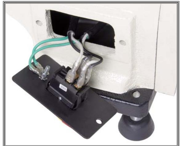
Figure 28. Switch connections.
