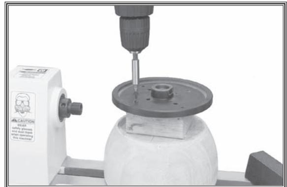
**Figure 24.** Typical example of mounting faceplate to a backing block.
