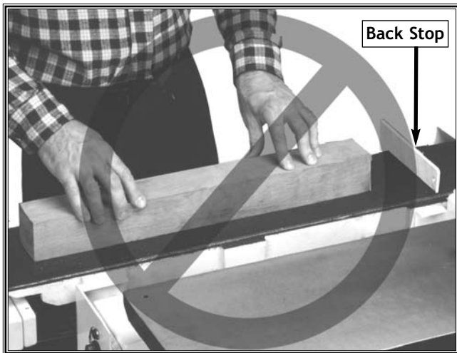
Figure 51. Incorrect face sanding away from back stop.
