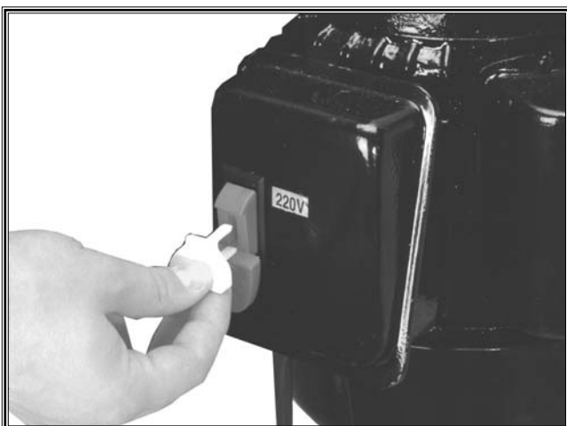
Figure 42. Safety lockout key removed.
