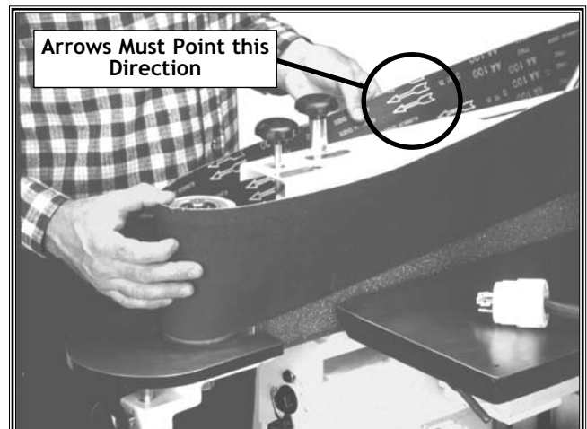
Figure 22. Sanding belt directional installation.
