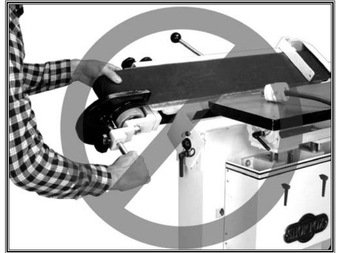
Figure 43. Incorrectly holding and tilting the platen.
