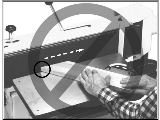
Figure 48. DO NOT sand wood with sharp corners at the leading-edge of the sanding operation. The belt can grab and throw the wood.
