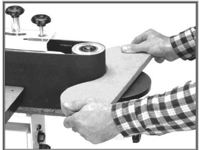
Figure 4. ALWAYS keep your fingers away from the idler roller and the belt.
