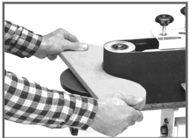
Figure 55. ALWAYS keep your fingers away from the idler roller and the belt.
