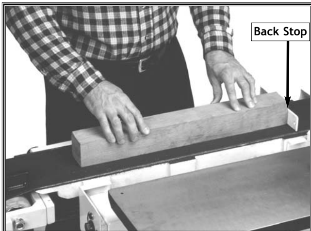
Figure 52. Correct face sanding.
