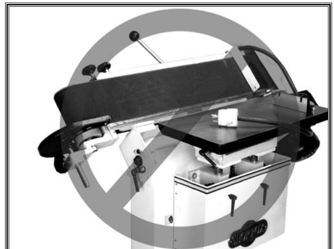
Figure 45. Incorrect platen tilted position.
