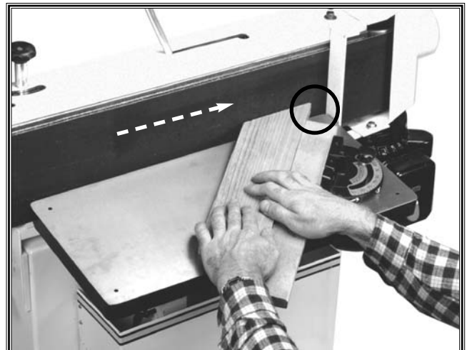
Figure 6. ALWAYS sand wood with sharp corners at the trailing-edge of the sanding operation.
