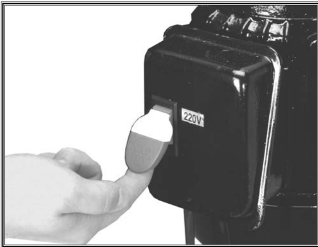
Figure 40. ON/OFF switch in the ON position.
