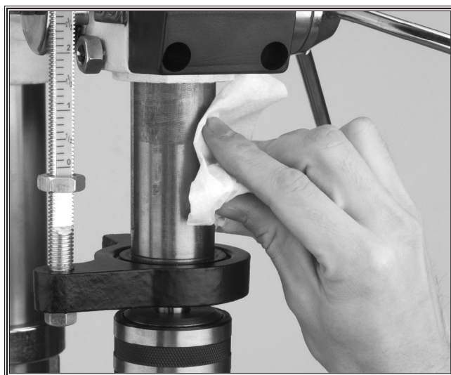
Figure 25. Clean and oil quill shaft.
