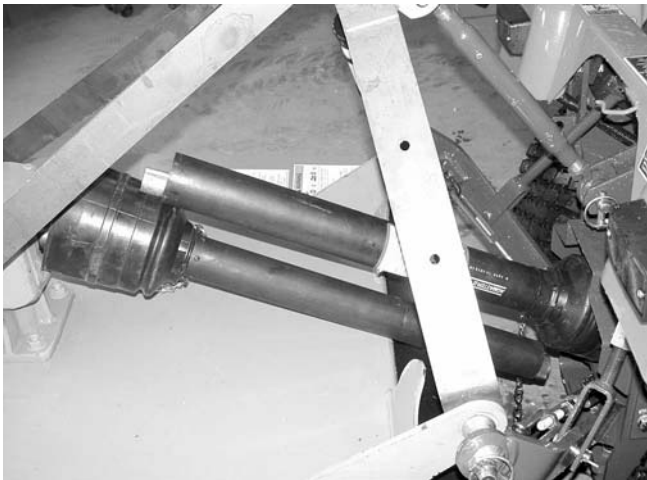
Figure 1. Drive Halves Placed Parallel
