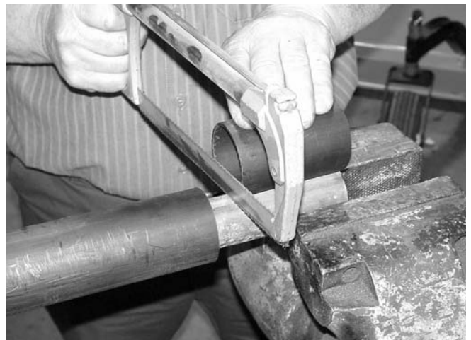
Figure 4. Cut Shaft to Length
