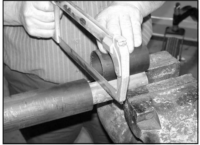
**Figure 6.** Cut Shaft to Length
