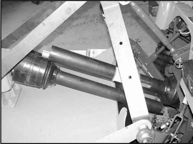
**Figure 3.** Drive Halves Placed Parallel
