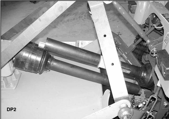
**Figure 5.** Drive Halves Placed Parallel
