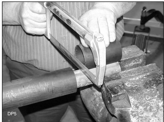
**Figure 8.** Cut Shaft to Length
