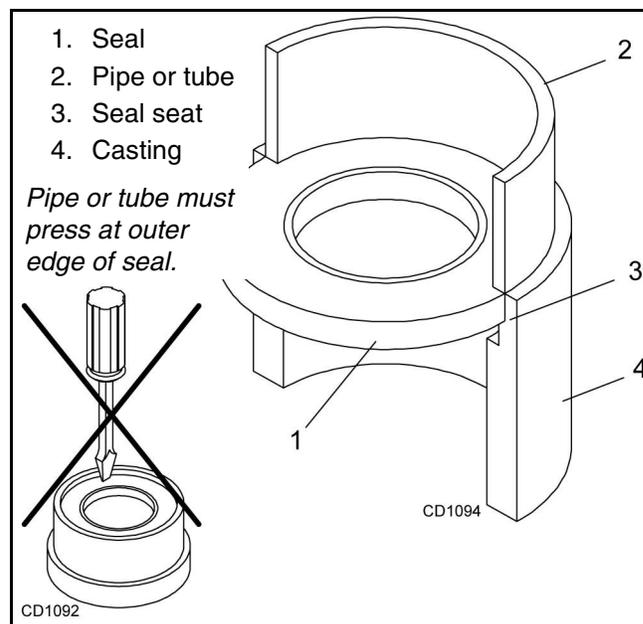
Figure 17. Seal Installation
