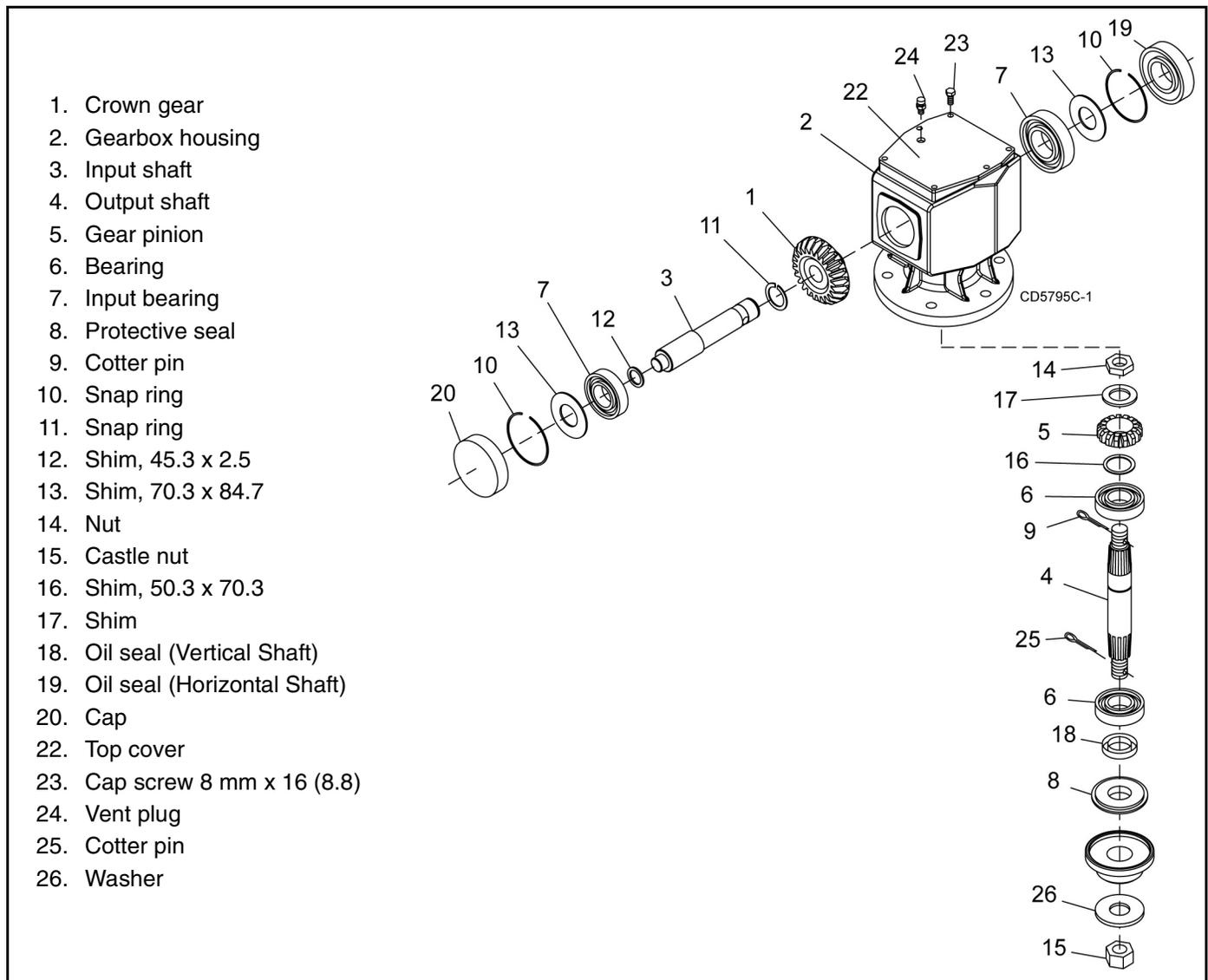
Figure 18. Gearbox Assembly
