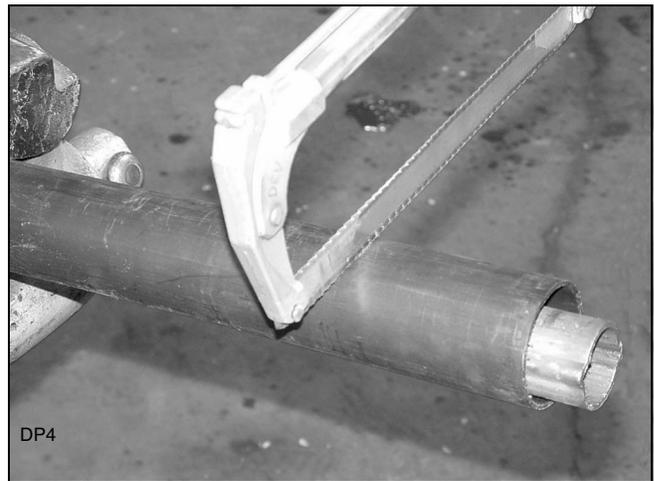
**Figure 7.** Cut Shield
