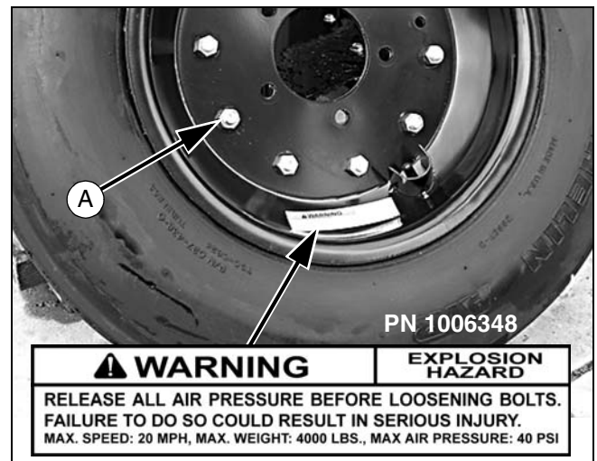
Figure 8. Split Rim Tire Servicing
