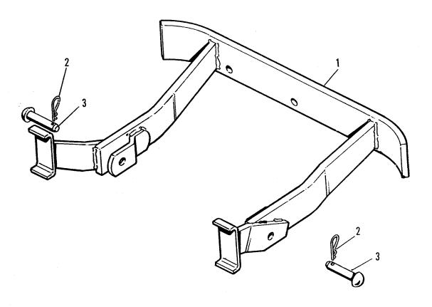
The front bumper is helpful in protecting the front end of the tractor from damage. The bumper is also required in order to mount the front counterweight (Not shown here).
