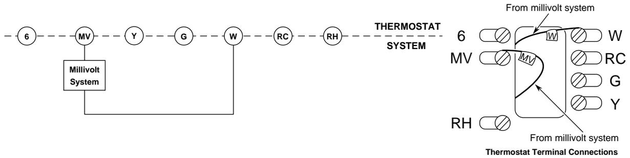
Figure 8. Typical Wiring Diagram for Millivolt Systems
