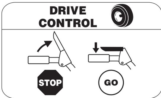
The drive control is located on the right handle. Squeeze the control grip against the handle to engage the wheel drive. Release to stop.
