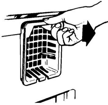
**To remove and replace the air freshener compartment.**
