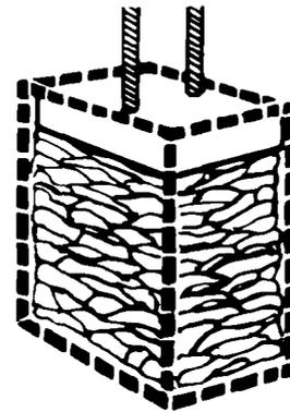
The trash in a full compactor bag will be about  $\frac{1}{4}$  the size of its original bulk.
