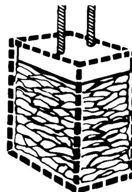
The compacting ram does not go to the drawer bottom. You will not see compacting of the first few loadings.
