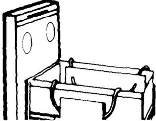
Fit the bag caddy in the drawer. Tuck the rope handles behind the bag retainers as shown.
