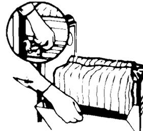
Push side-lock lever down and tilt drawer side open.
