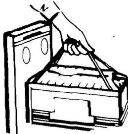
Remove bag carrier handles from side retainers and hold.
