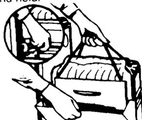
Push side-lock latch down and tilt drawer side open.
