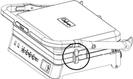
A line drawing of the Versagrill appliance in its closed, horizontal position. The storage clip on the right side is now closed, with its handle pointing inwards. A circle highlights the clip's mechanism. |
