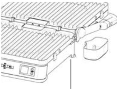
Locate the grease cups onto the locating pins as shown.
