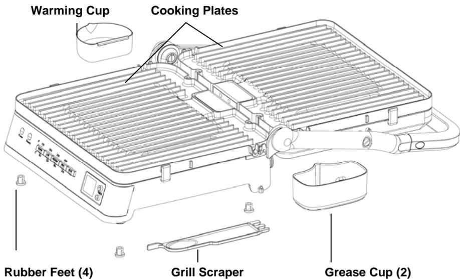
**Cooking plates:** The removable and reversible, upper and lower cooking plates are interchangeable. The cooking plates are reversible with a grilling surface, ribbed on one side and a griddle surface, flat on the other side. Both cooking plates have a non-stick surface for easy cleanup.
