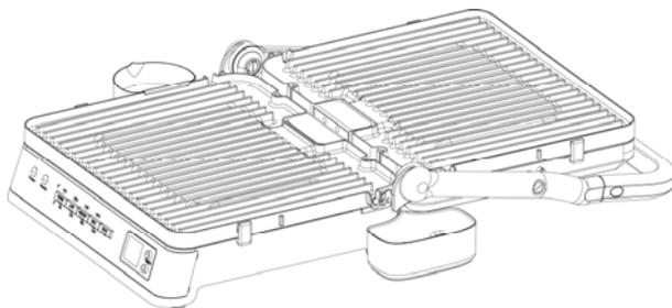
**Warming/Buffer Operation:** To use the appliance in a warming buffet scenario, open the top cooking surface all the way until the handle is resting on the counter. The cooking plates need to be in place with both grill surfaces up. Most any stove top pan, foodservice pan, or baking pan, must be high temperature capable, can be set on the surface to keep the contents of the pan warm.
