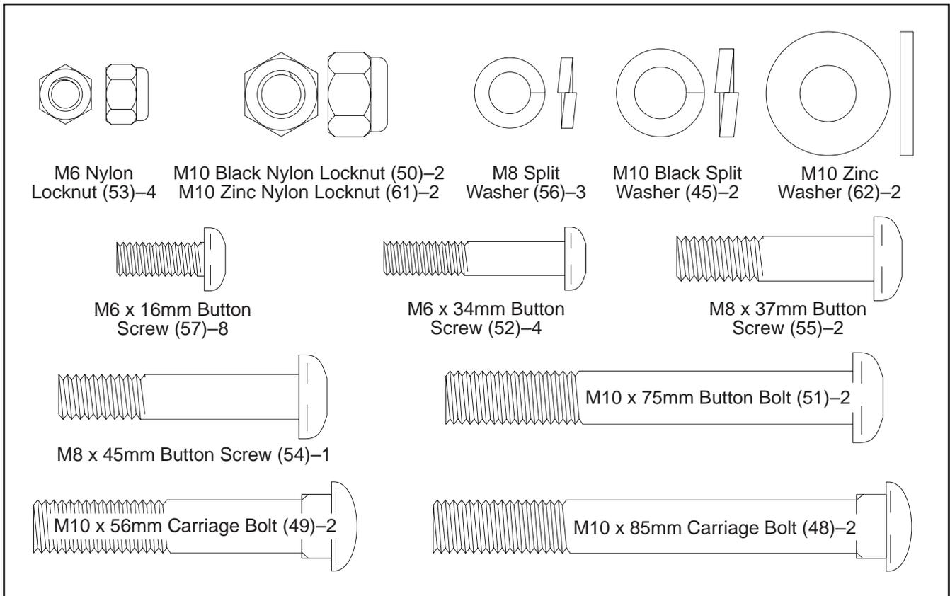
1. Identify the Front Stabilizer (2). Turn the Front Stabilizer so that the warning decal is in the position shown. While another person lifts the front of the Frame (1) slightly, attach the Front Stabilizer to the Frame with two M10 x 85mm Carriage Bolts (48) and two M10 Black Nylon Locknuts (50).
