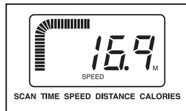
3. To reset the display, press the mode button for two seconds. After the display is reset, the scan mode will be selected.
