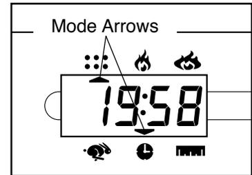
Speed, time, distance, fat calories, or calories mode—To select one of these modes for continuous display, press the mode button repeatedly. The mode arrows will show which mode is selected. Make sure that the scan mode is not selected.
