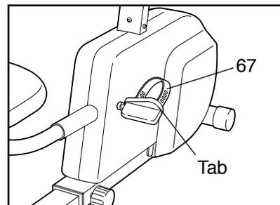
Press the Pedal Strap onto the adjustment tab. Adjust the left Pedal Strap (not shown) in the same way.
