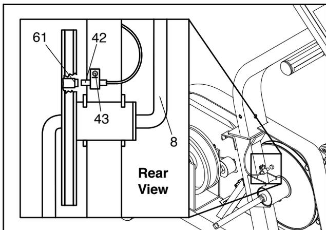
With the left side shield removed, locate the Reed Switch (42). Turn the Crank (8) until the Magnet (61) is aligned with the Reed Switch. Loosen, but do not remove, the M4 x 16mm Screw (43). Slide the Reed Switch slightly closer to or farther away from the Magnet. Retighten the Screw. Turn the Crank for a moment. Repeat until the console displays correct feedback. When the Reed Switch is correctly adjusted, reattach the left side shield and the left pedal.
