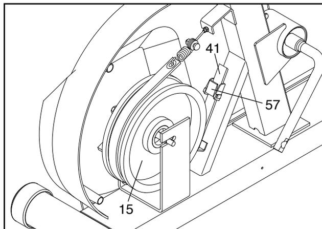
With the left side shield removed, turn the resistance knob to the lowest setting (see HOW TO ADJUST THE PEDALING RESISTANCE on page 9). Open the Strap Clamp (57) and pull the end of the Resistance Strap (41) slightly upward to increase resistance. Close the Strap Clamp and turn the Flywheel (15) to make sure that there is not too much resistance. When the Resistance Strap is properly adjusted, reattach the left side shield and the left pedal.
