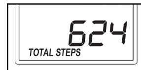
To reset the display, press and hold down the Program Start/Reset button for a few seconds. The display information will then be reset.
