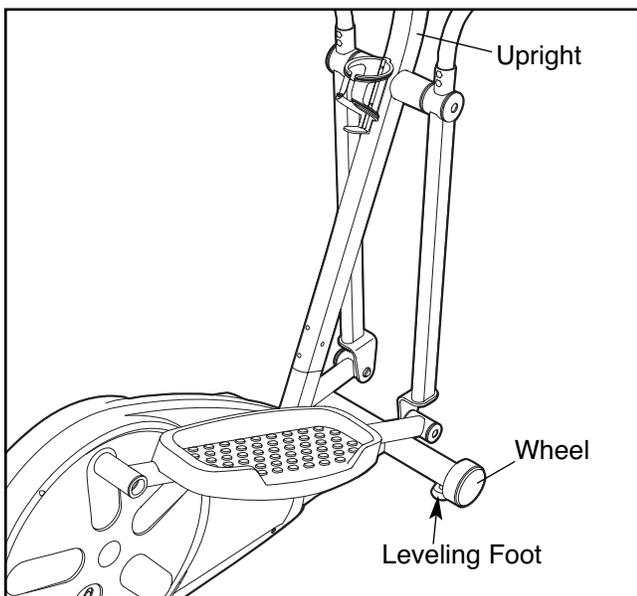
If the elliptical exerciser rocks slightly on your floor, turn one or both of the levelling feet under the front stabilizer until the rocking motion is eliminated.
