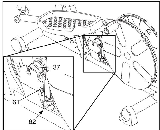
Next, loosen the M8 x 19mm Flat Head Bolt (61) and turn the Adjustment Screw (62) until the Belt (37) is tight. Once the Belt is tight, tighten the Flat Head Screw. Then, reattach the side shields. Note: If you have questions as to which screw should be in which hole, see EXPLODED DRAWING B on page 19 and the PART LIST on page 17.
