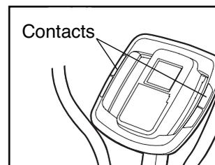
**Avoid moving your hands or gripping the contacts too tightly.** When your pulse is detected, a heart-shaped symbol will flash in the display each time your heart beats and then your heart rate will be shown. For the most accurate heart rate reading, hold the contacts for at least 15 seconds. Note: If you continue to hold the handgrip pulse sensor, the display will show your heart rate for up to 30 seconds. The display will then show your heart rate along with the other modes.
