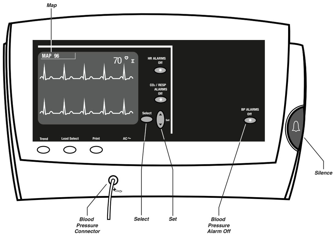
**Atlas Monitor waveform display showing location of MAP reading**
