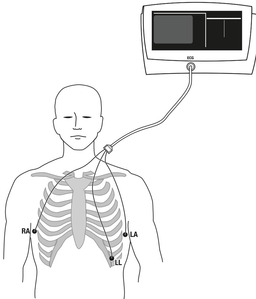
**Alternate ECG electrode placement for Impedance Respiration**
