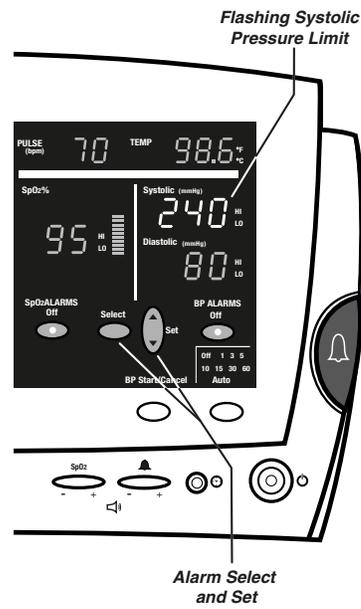
**Atlas Monitor showing alarm setting displays and controls**
