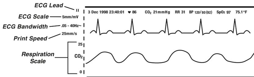
**Atlas Monitor showing waveform display and printed waveform record**
