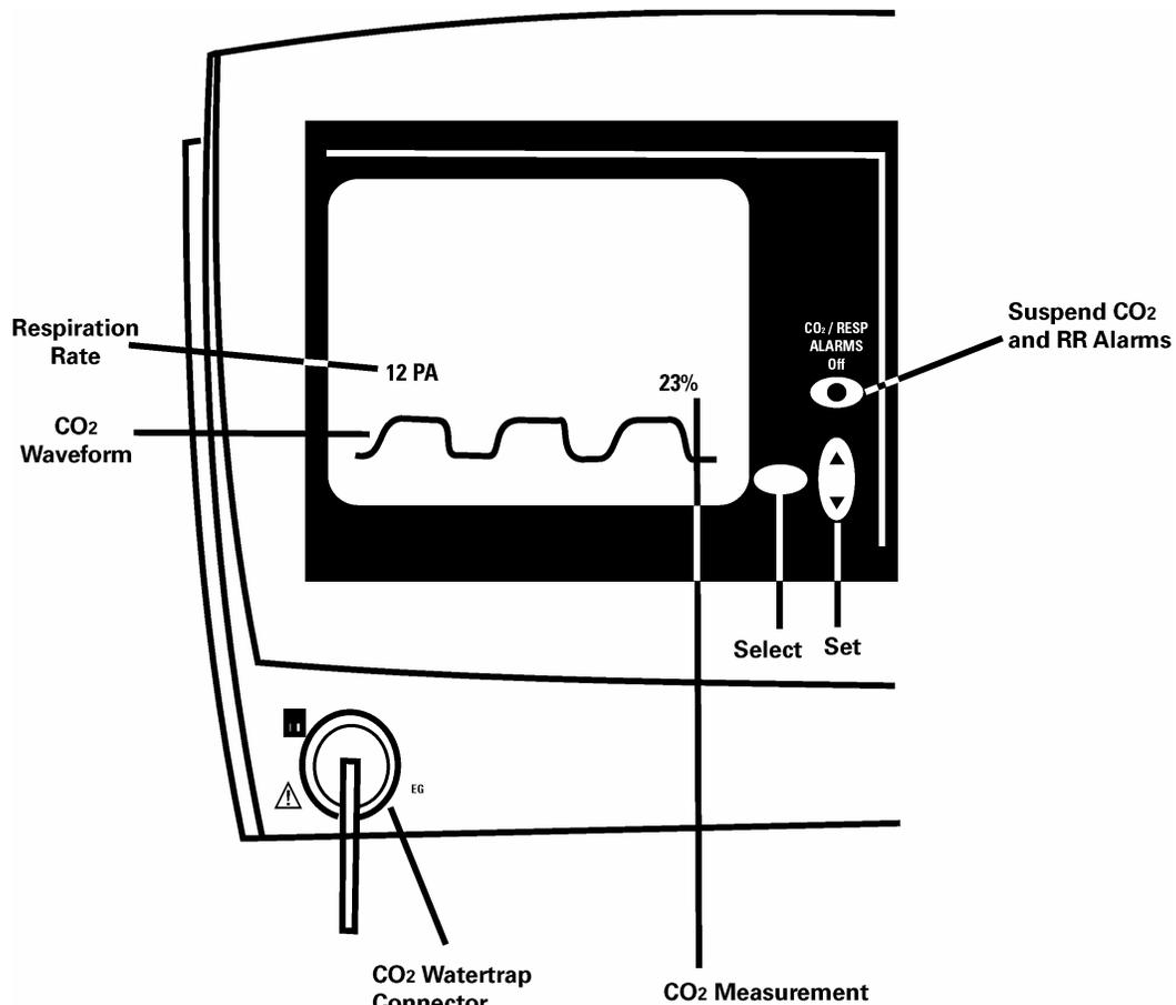
**Atlas Monitor model 623xx showing ETCO<sub>2</sub> waveform display, controls, and watertrap connector**
