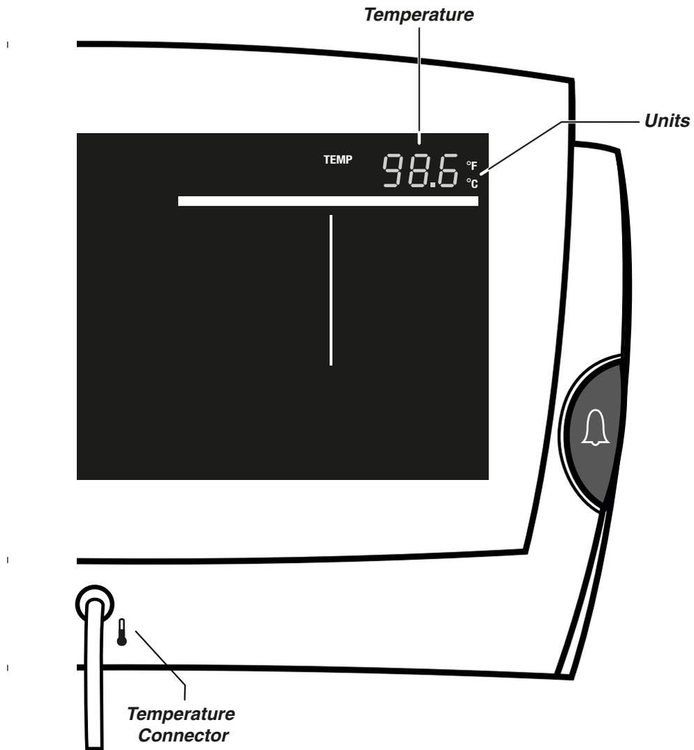
**Atlas Monitor showing Temperature display and connector**
