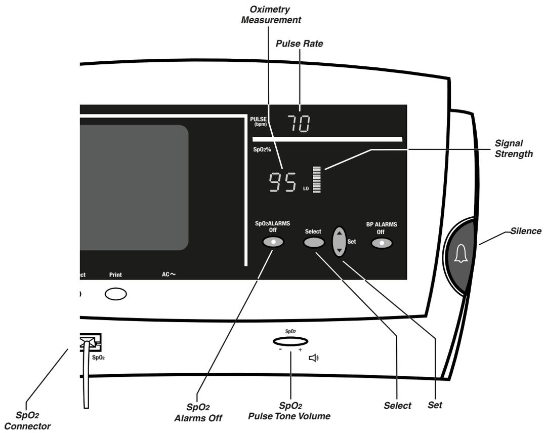
**Atlas Monitor showing SpO<sub>2</sub> displays, controls, and sensor connector**
