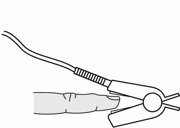
Correct placement of reusable Nellcor SpO<sub>2</sub> fingerclip sensor
