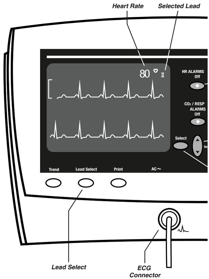
**Atlas Monitor showing ECG waveform display, controls, and ECG connector**
