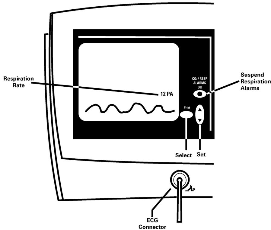
**Atlas Monitor showing Impedance Respiration waveform display, controls, and ECG connector**
